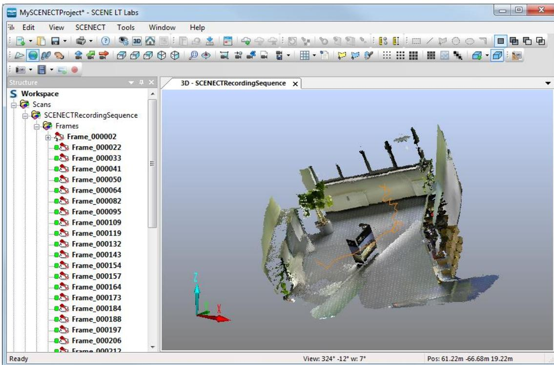
**Figure 3-2: 3D view of a sequence**
