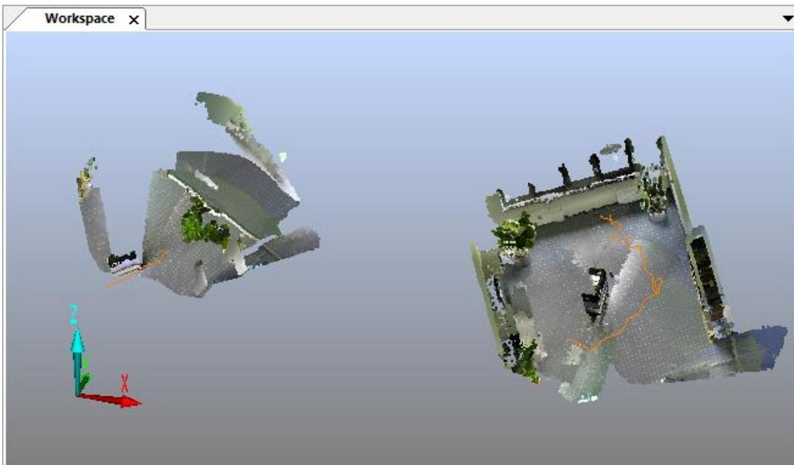
**Figure 3-6: Not registered sequences in 3D view**
