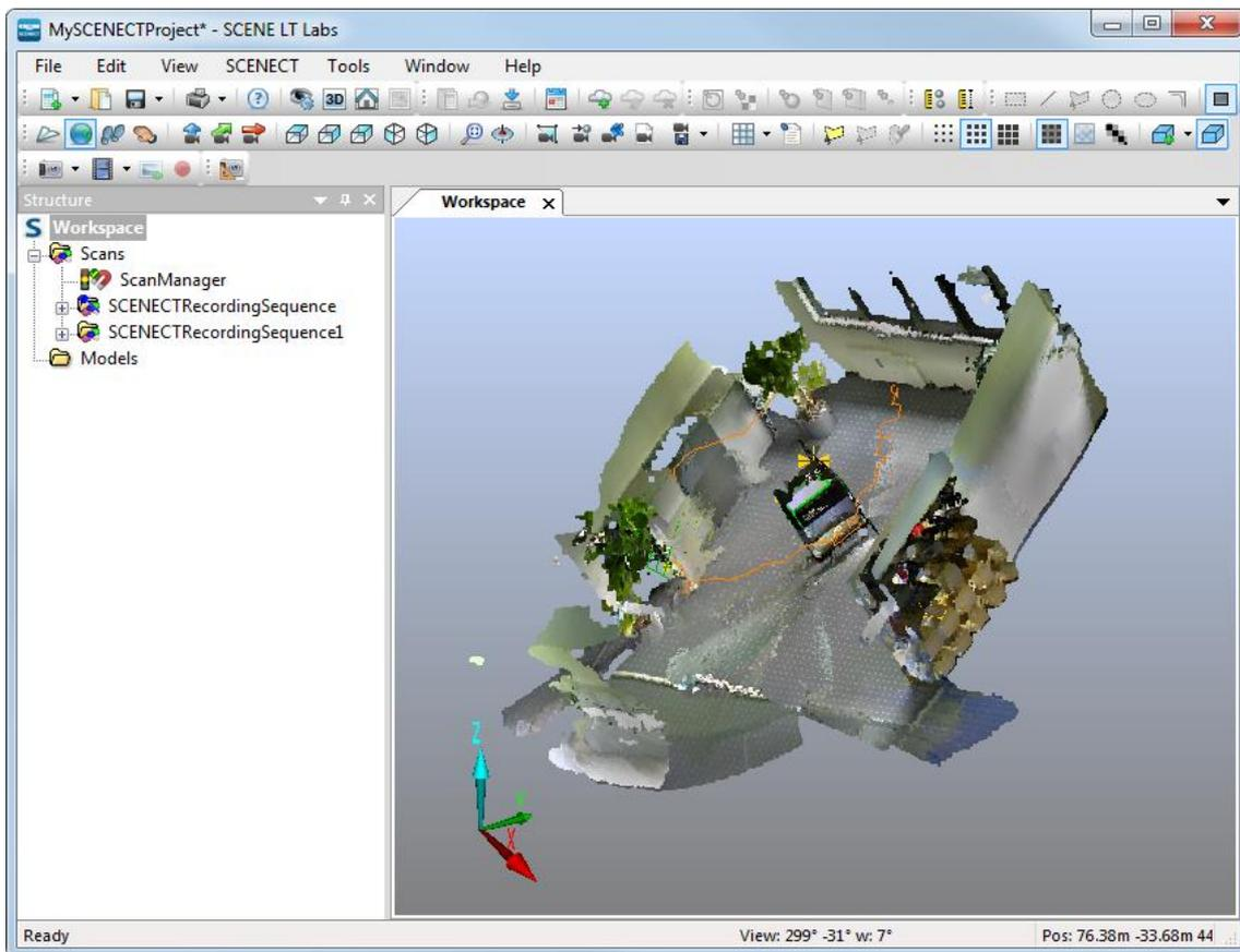
**Figure 3-14: Registered sequences in 3D view**
