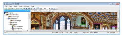
Figure 3-12: Scan point data in the status bar
