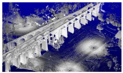
Figure 3-11: Initial scan alignment of project after import
