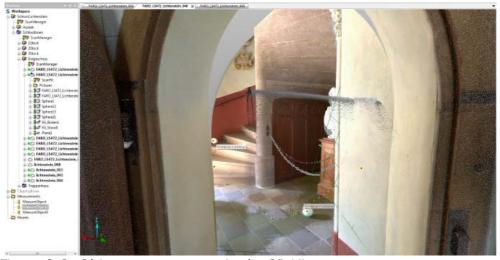
Figure 8-8: Object measurement in the 3D View
