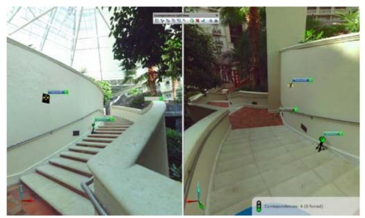
Figure 6-10: Correspondence Split View with automatically detected targets
