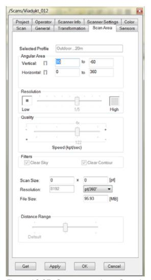
Figure 16-97: Scan properties - Scan Area
