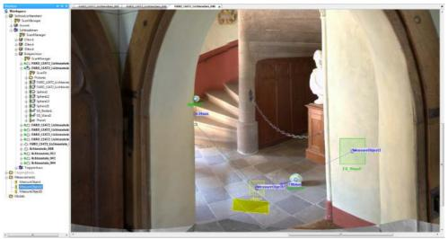
Figure 8-7: Object measurement in the Planar View
