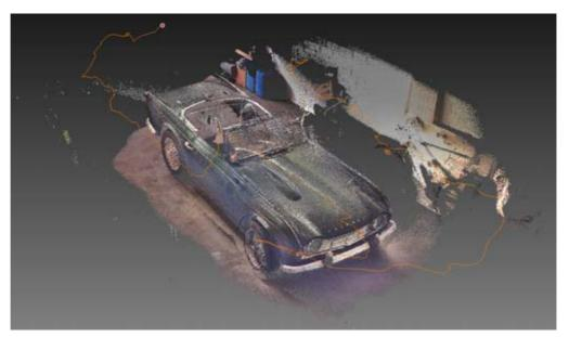
Figure 7-52: 3D View of a scan, the scan path is displayed
