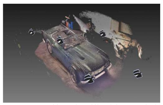
Figure 7-54: 3D View of the VirtualScans folder with the positions of each virtual scan
