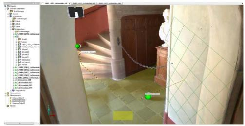
Figure 8-6: Object measurement in the Quick View
